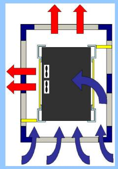
By using a range of modular components including our vertical brush strips, quick fit 19-inch blanking and these fixed side blanking plates users can quickly and easily configure an Access Cabinet to manage active equipment having air flow cooling requirements other than conventional front to back aspiration.
